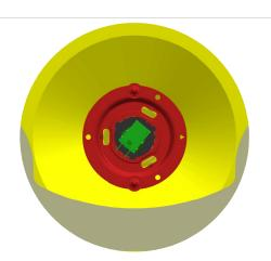
2. Insert By Aligning Switch Bracket with Receptacle
