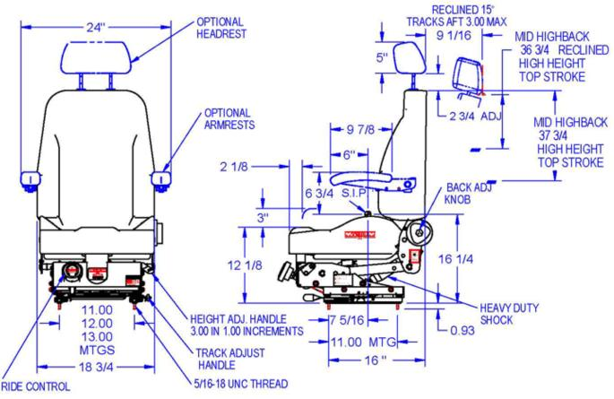
\*OPTIONAL FIELD ADJUSTABLE TRACK MOUNTINGS 11.00", 12.00" & 13.00". NOTE: Proper length tie-wire must be ordered when modifying track mounting.
