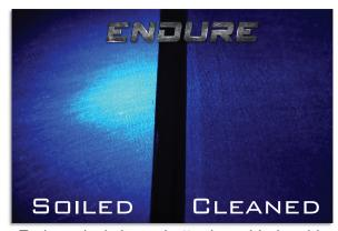
Endure vinyl cleans better in a side-by-side comparison of materials. Sample shown was soiled with glo-germ and then cleaned with soap and water.
