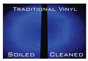
"Standard" vinyl performance. All samples were subjected to the same level of soiling and cleaned with the same soap and water to maintain a baseline for comparison.
